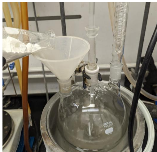
Add in a single portion, and raise temperature to 70- 73 °C
