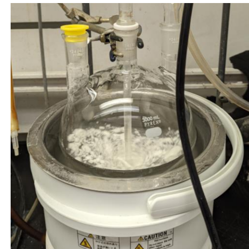
Starts off as a suspension with large particles. Increase the speed of the mechanical stirrer
