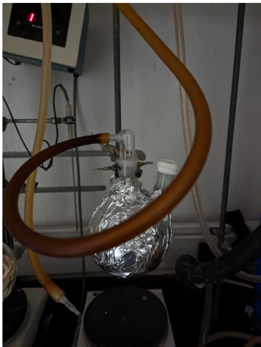
With all the solvent removed leave on the high vac over night.
