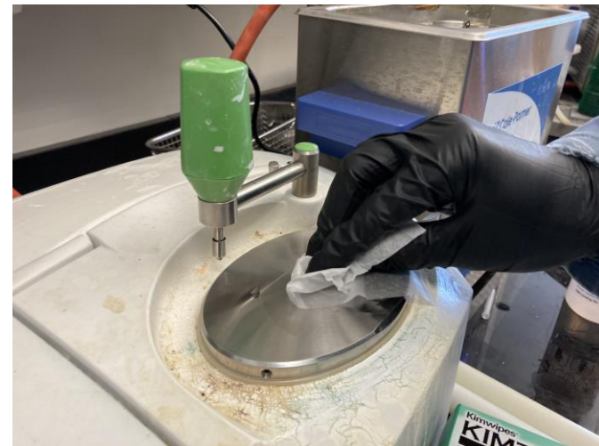
12. Wipe off surface of detector with acetone and kim wipes
