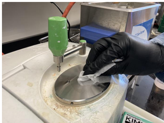
2. Wipe off surface of detector with acetone and kim wipes
