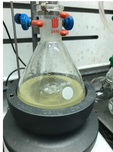
3. Gradually open the system to vacuum so that solvent bubbles gently
