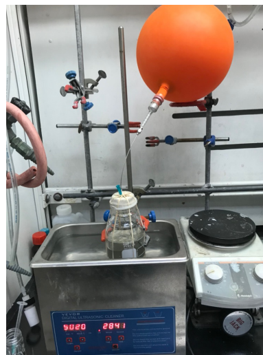
4. Sparge with argon while sonicating for 30 min
