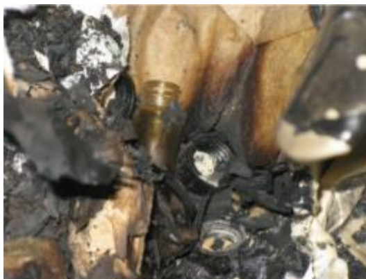
Figure 14. Catalyst fire during filtration.
